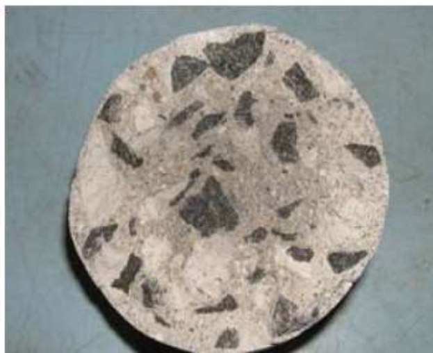
Concrete exposed to CO 2 (accelerated test)
